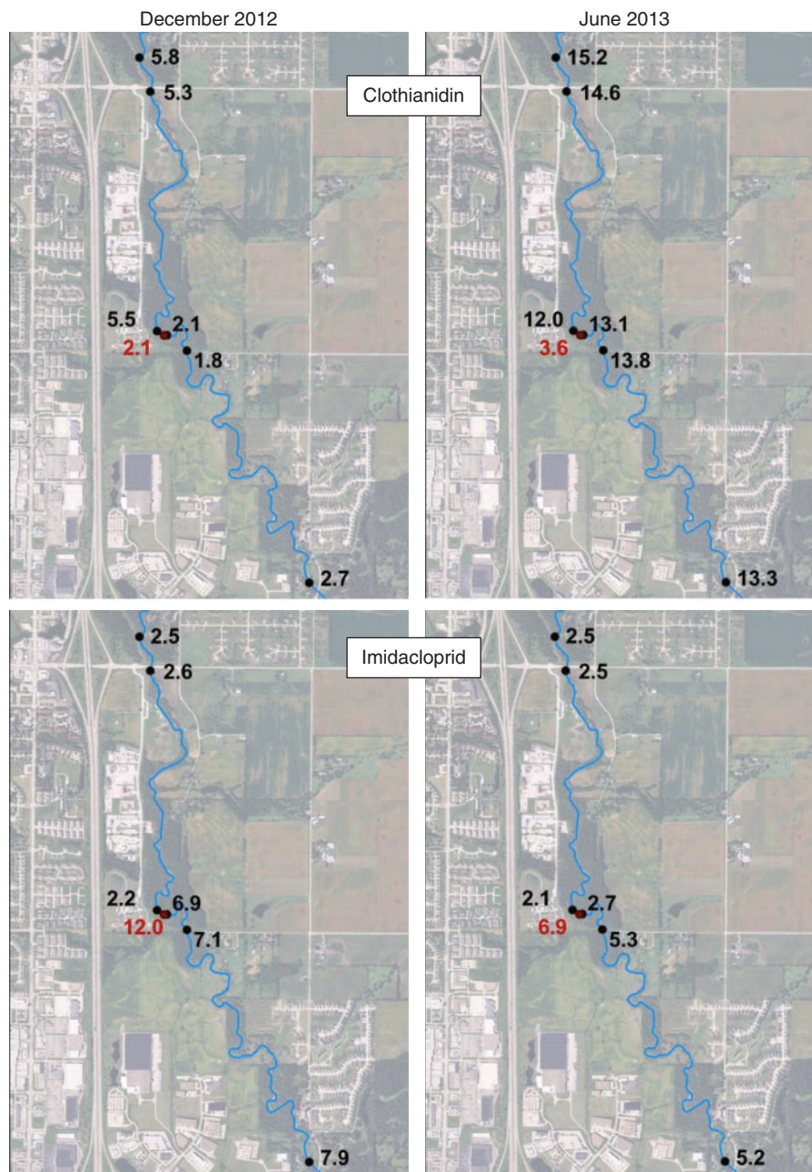
Fig. 7. Concentrations ( \text{ng L}^{-1} ) of clothianidin and imidacloprid collected along Fourmile Creek near Ankeny, Iowa, at two sampling times, December 2012 and June 2013. The concentrations in red are those found at the outfall of the wastewater treatment plant (WWTP).
