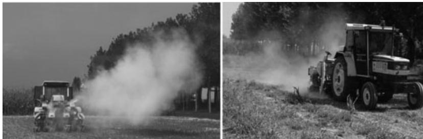
**Fig. 2** Visual image, obtained by introducing talc into the hopper, of the cloud emitted by an unmodified drill (left) and a drill with dual-pipe equipment (right). The modification pushes the cloud closer to the ground but is still consistent.
